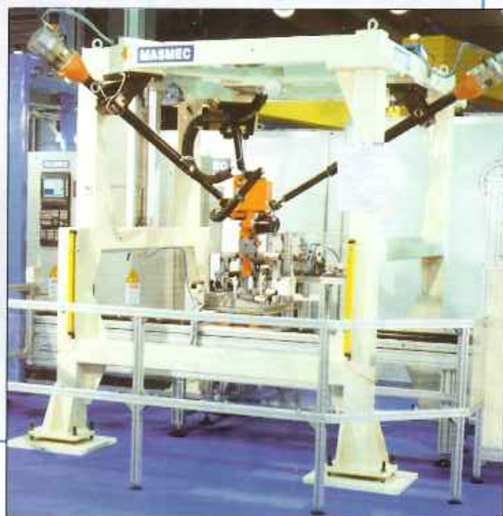
▲ Fig. 1 La Ipkm (Industrial parallel kinematic machine) italiana
